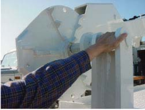
Example of stow mechanism pin being positioned into TireHand pad - street side.
