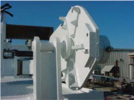
Full engagement of stow mechanism pin in TireHand pad.
